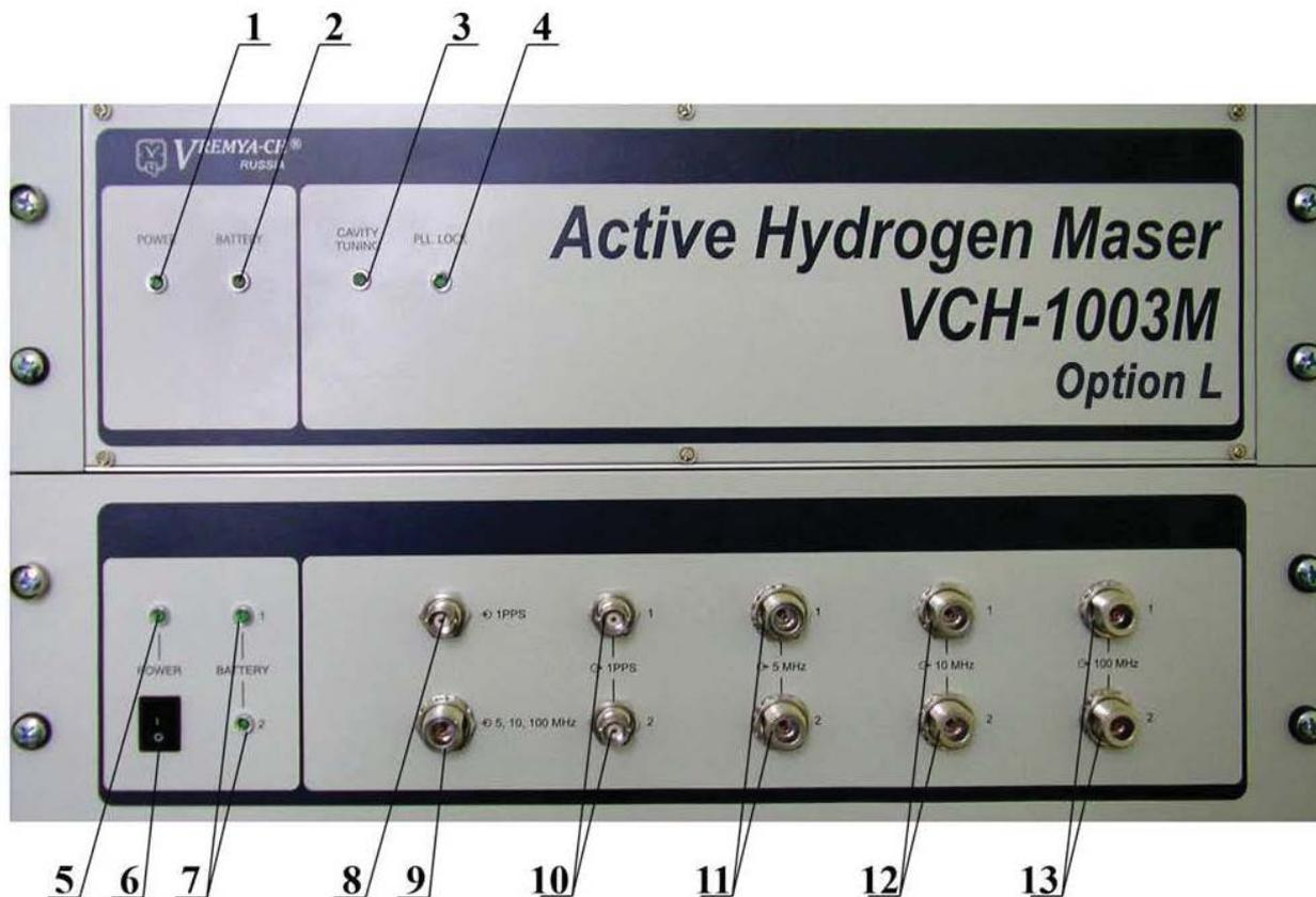
Figure 7 Indicators, connectors and switches on the maser’s front panel
