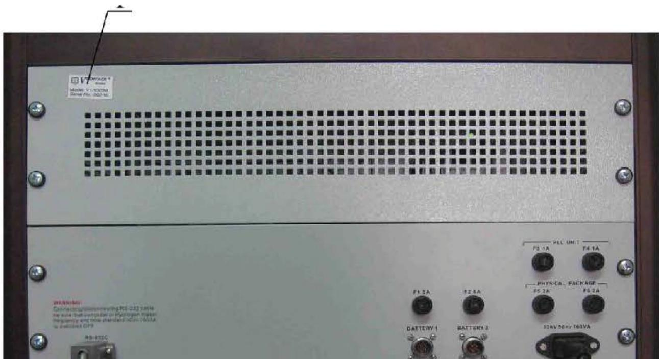
Figure 10 Serial number and production date label
