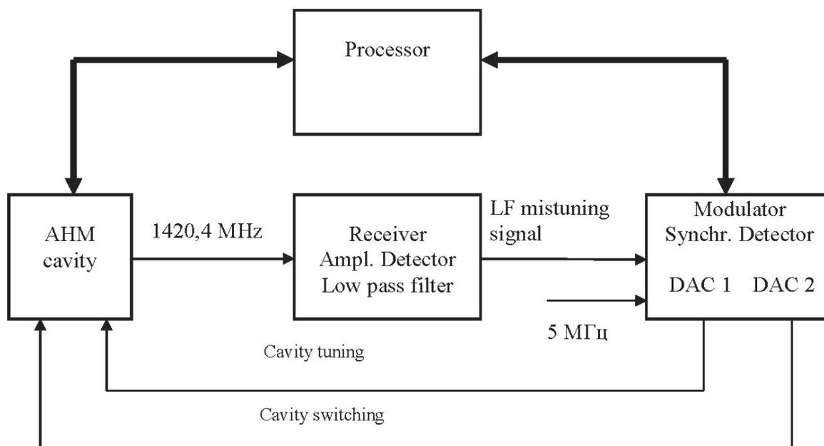
Figure 5 Cavity tuning system
