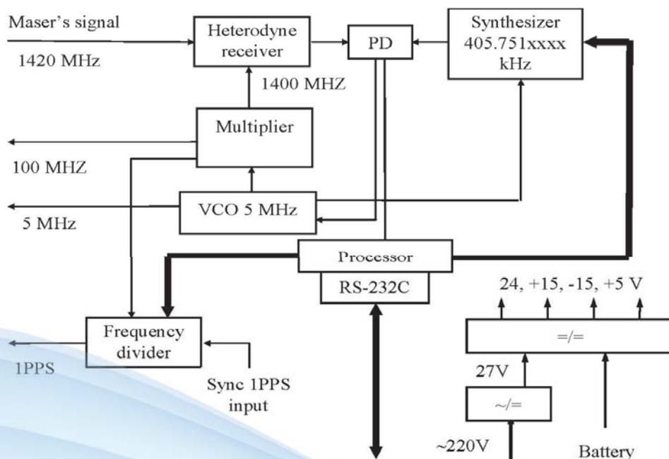
Figure 4 PLL Unit circuit
