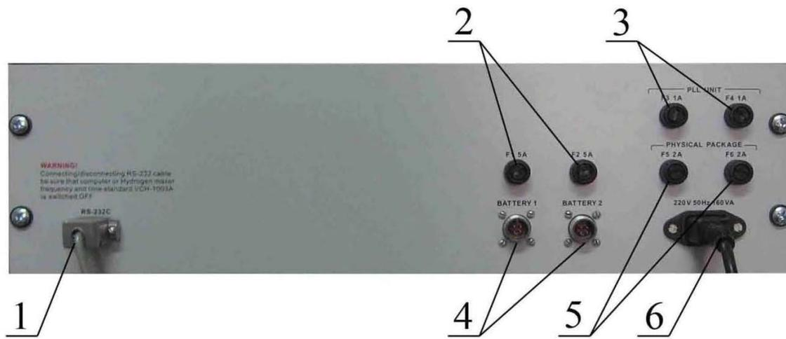
Figure 8 Connectors and switches on the maser's rear panel
